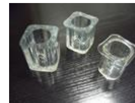
Thick section produced by overmoulding in 3 stages
