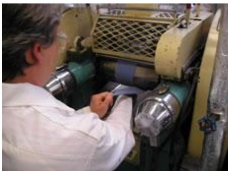
Mill mixing of a rubber compound
