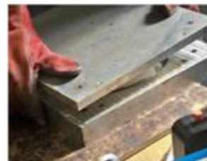
Loading the Frisbee mould with recycled milk bottles
