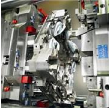
4 station rotating mould for 3-component moulding (one stage for ejection)
